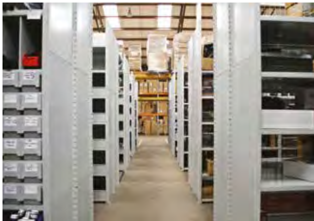
Cross aisles help cut down journey times in picking operations, which helps increase efficiency and keeps fire escape routes clear.
