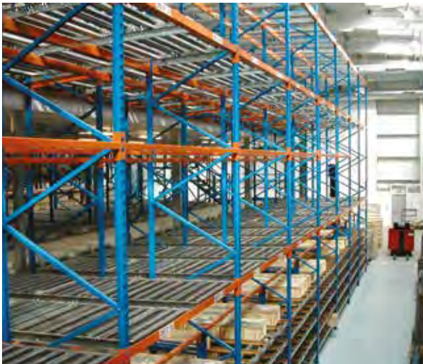
Pallet live can be used to feed multi level picking operations, where pallets are broken down for picking.
