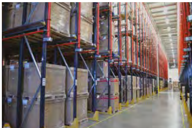
Pallets are stacked by the first-in, last-out (FILO) principle, which means that individual pallets cannot be accessed directly, but one by one from the front face of the rack.
