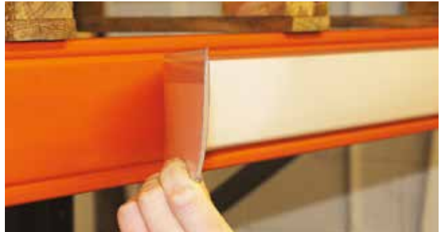
Self adhesive strip runs along the back of the plastic holder
