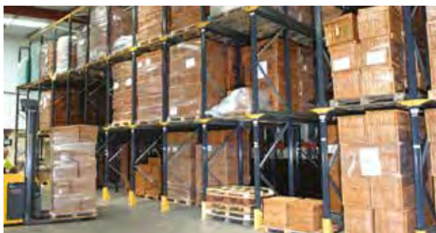
With limited stock rotation, Drive-in pallet racking is particularly suitable for seasonal goods.
