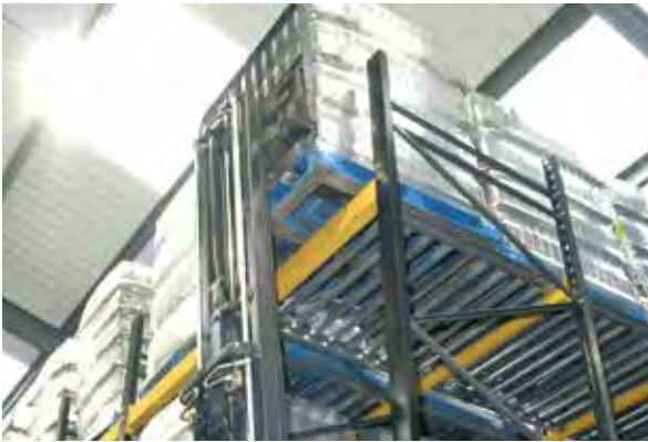
Push-back racking allows for the storage of up to 10 pallets deep.
