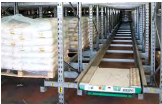
The length of the storage lane is not limited in the same way as a pallet live system, with no incline required.
