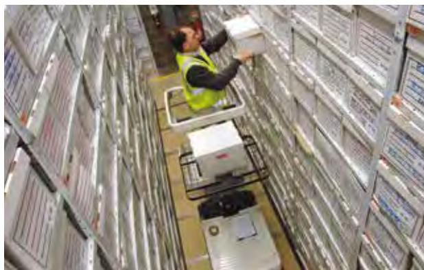
Mechanical access equipment allows for higher shelving to be considered, utilising the full building height.
