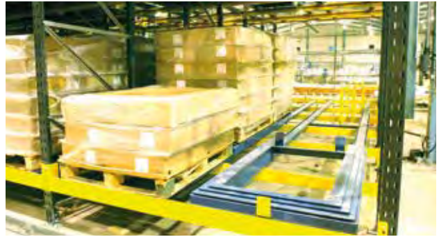
Pallets are loaded onto wheeled carts or rollers, and are pushed back along inclined beds. When a load is retrieved, the remaining pallets roll forward into position at the picking face.
