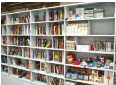
Shelf dividers are used to create 'pigeon holes' in these clad Stormor bays. These are adjustable along the shelf width.
